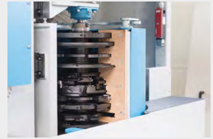
Chip breaking device for tenoning
