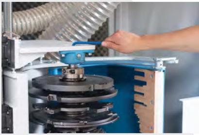
Innovative change system for tenoning tools
