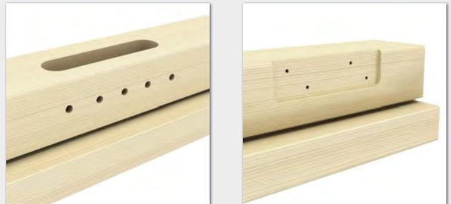
Longitudinal milling and drilling
