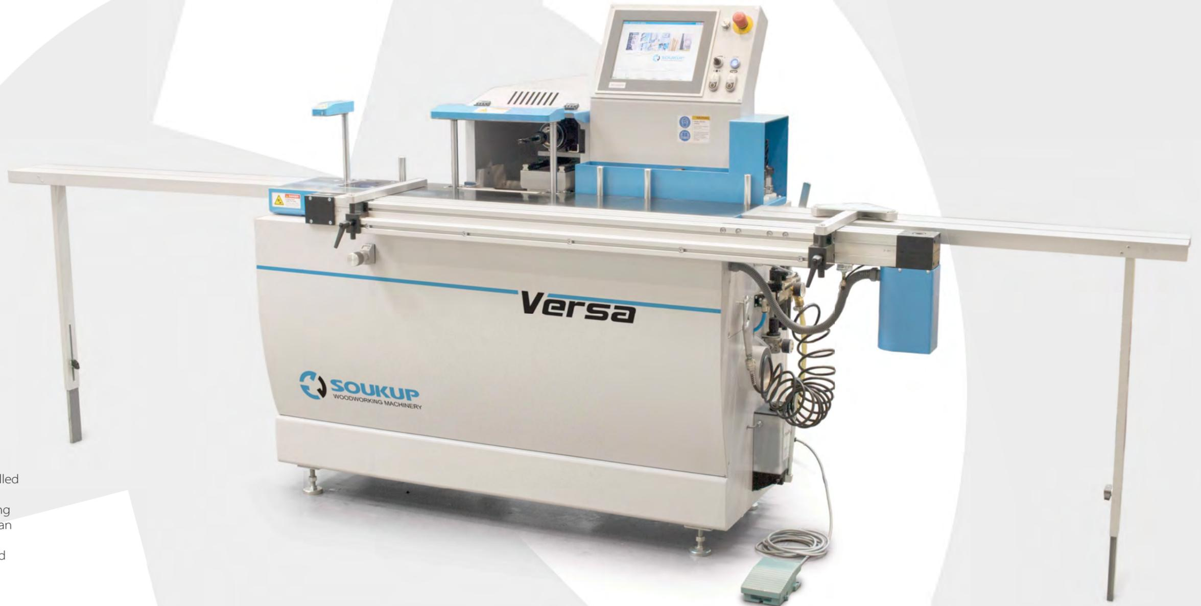
The machine allows you to drill holes for dowel connections or mortise slots. The lateral NC controlled working unit has 3-axis and allows drilling to any schema and mortising slots for tenons. Additionally, you can do door lock pocket milling, hinge seats, bevelled louvres mortises and front rounding of tenons.
