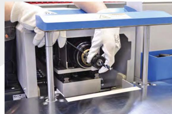
Milling of bevelled slots and tenons
