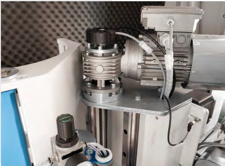
Electronic positioning of the tenoning unit
