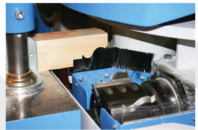
Horizontal milling unit for heritage sash horn detail or trenching of sash box
