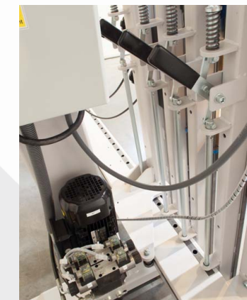
Hydraulic pump – self locking pins
