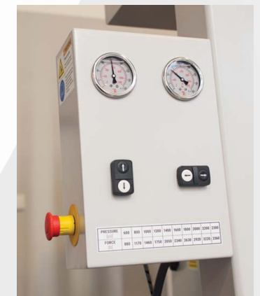
Two pressure gauges for vertical and horizontal direction
